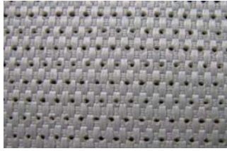
Fig. 3 Fabric detail with the holes of 0,4 mm diameter.
